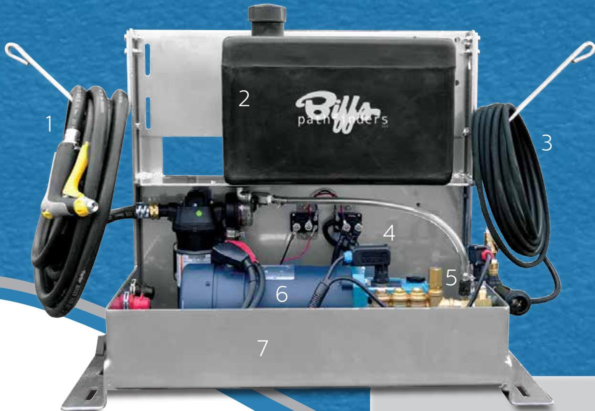
Operating and maintaining the Pathfinders spray system takes very little time and is easily serviceable due to its compact design. A highly dependable 1250 psi pump, with auto-shut off and adjustable flow rate, is the power behind dual spray guns. One gun operates at 5 GPM for charging the tank, while the other functions as a high-pressure sprayer for cleaning or low pressure sprayer for applying the disinfectant.
